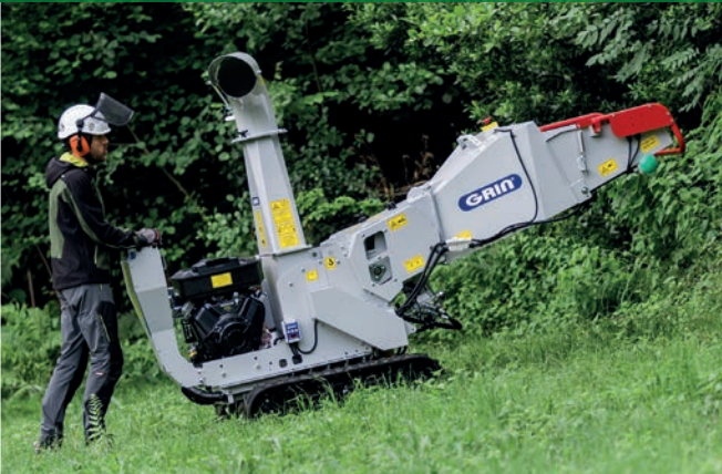
03. SINGLE ENGINE TO SHIFT THE CENTER OF GRAVITY DOWNWARDS
